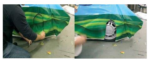
In a single smooth arched movement, the vinyl that is covering the wheels can also be cut away, taking care not to cut too much off, so that it can be fitted snugly into the wheel arches.
