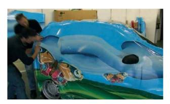
When you start applying the vinyl over the upper part of the vehicle, you also have to heat the vinyl over the biggest possible surface (in order to divide the elongation and not to create too much tension on a small piece of vinyl), and then pull it over the border.
