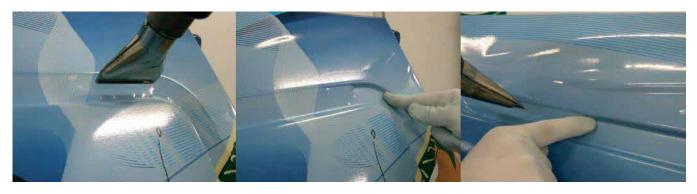
Now the opposite edge can be applied on the outer side. The inner side of the groove needs to be heated, so you can press the outer side of the groove.
