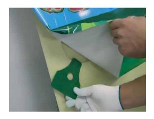
Before continuing application, place a squeegee between the surface and the print, so that the air can escape while pressing the vinyl. First start pressing the vinyl at the inner side of the indentation!
