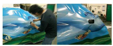
First make sure that a hole/slit is cut at outside mirror height. Care should be taken not to make the hole/slit too big, or there will be insufficient vinyl to apply around the mirror.
