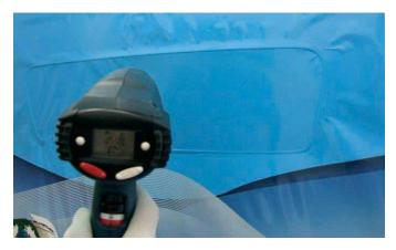
Always heat the vinyl at the bottom edge of the indentation, and press the vinyl gently into the indentation.
