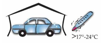
The ideal environment for wrapping is a well illuminated, dust free area with a constant temperature between 17°C and 24°C. The vinyl used should also have acclimatized sufficiently. The preparation of the vehicles includes the removal of number plates, window rubbers, mirrors, the antenna, etc...
