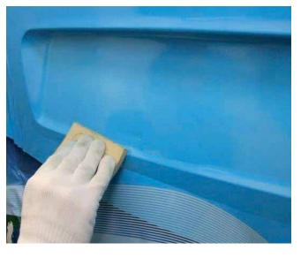
The middle of the section of vinyl can now be easily pressed in by means of the felt squeegee. The superfluous air can easily be guided through the holes where the number plates are supposed to be attached.
