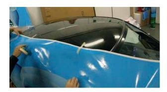
Secure the print to the roof by means of 2 pieces of tape. Cut the tape in half, and remove the backing paper completely.
