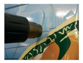
Once the air is pushed gently through the small incision, the area should be after-heated at 350°C (picture 4).
